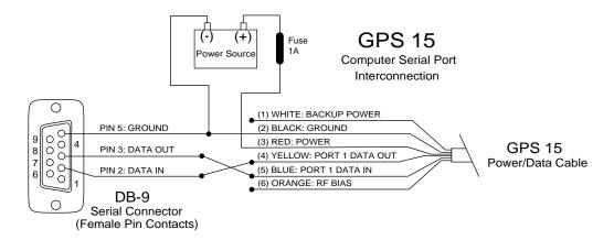
Figure 1. Computer Serial Port Interconnection
